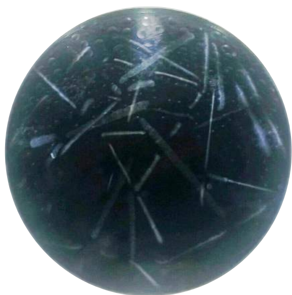
Tracks of \alpha particles from 220 Rn
